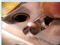
Repairing Chipped Edges
