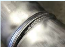
Tube Splicing Welding
