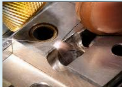
Mold Hole Repair
