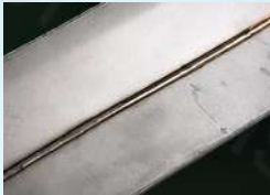
2mm Inside Fillet Weld
