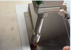
Reinforcing Rib Welding
