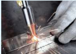
Stainless Steel Welding
